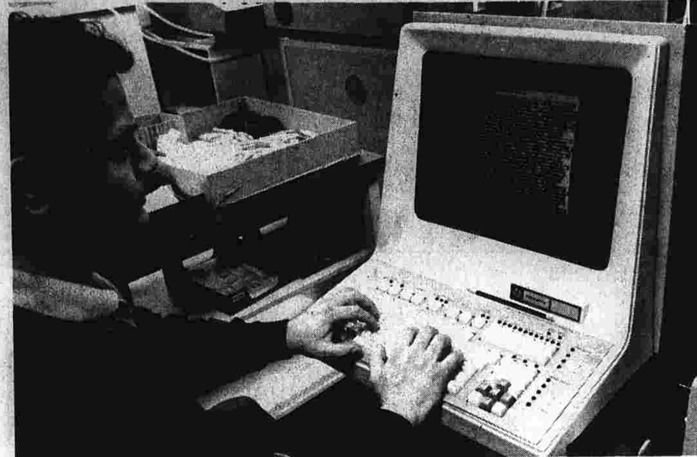
Proofing and editing in the composing room is accomplished with two Hendrix 5200 terminals. John Rosati, one of the operators, has the story in front of him on the video screen where he can add or delete words or lines. When he is satisfied the story is okay, he pushes a key which activates one of the Photon Facsetters and converts the paper tape into paste-up type.
