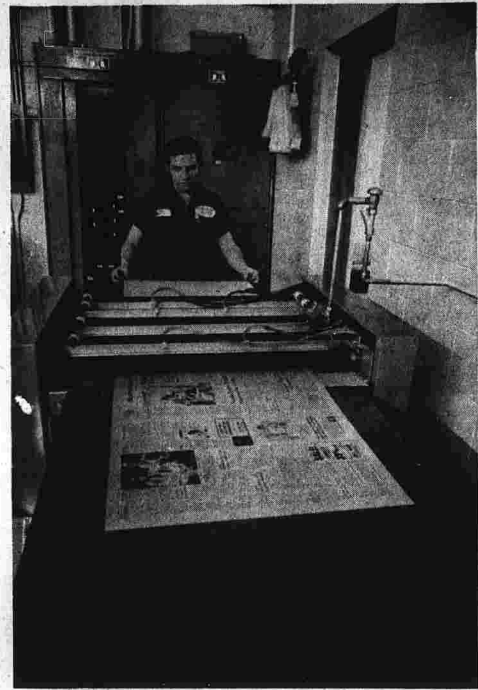
The work of developing the aluminum plate for the press is now done automatically. Previously it was accomplished by hand. Jim Adams feeds a plate into the National machine.
