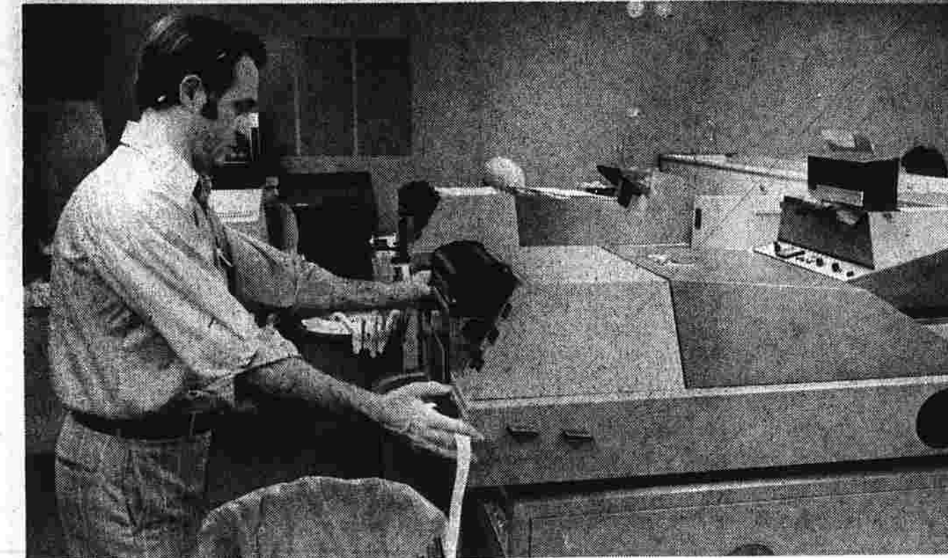
Sheldon Cohen feeds tape into a Photon 813 Facsetter which is capable of photographing news copy into paste-up type at the rate of 90 lines per minute. Type, ranging in size from 6 to 72 point, can be delivered from the Photon machines.
